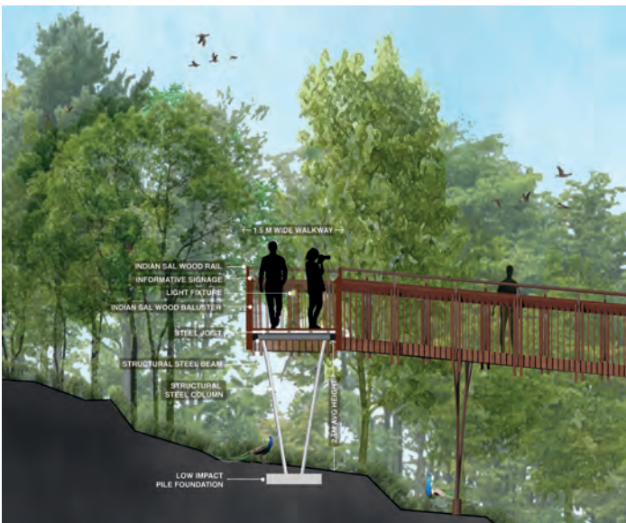
Malabar Hill Forest Trail – The elevated walkway will be constructed without damaging a single tree.
